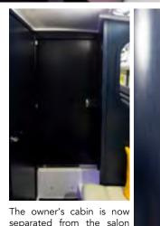
The owner's cabin is now separated from the salon by a sliding door. This space-saving solution creates a passage of maximum width.
